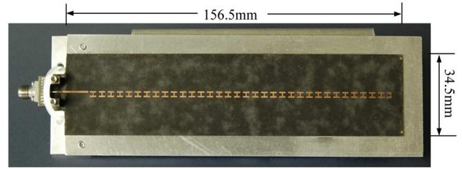
Fig. 8. Fabricated frequency-scanned leaky-wave antenna. A 2.92-mm end-launch connector is applied as the feeding port.
