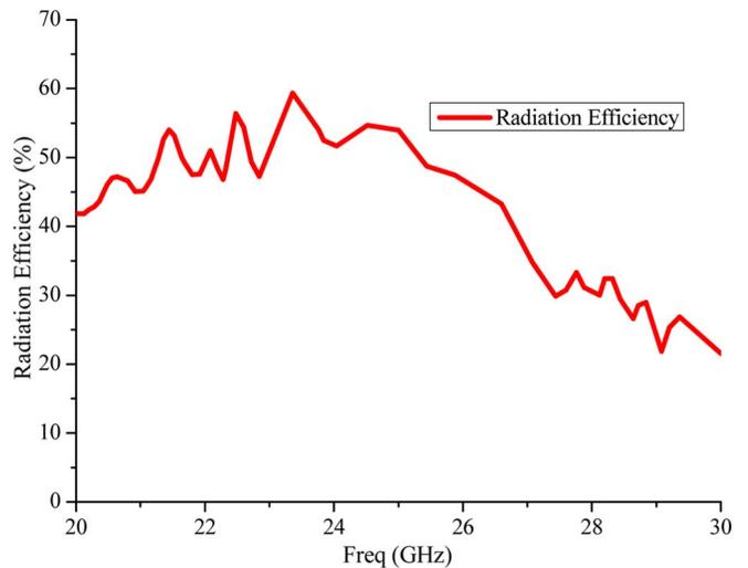
Fig. 10. Radiation efficiency of the leaky-wave antenna.
