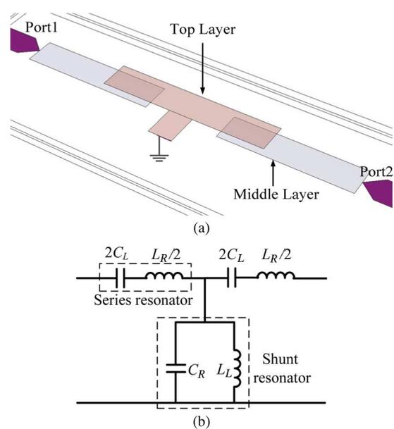
Fig. 5. (a) CRLH microstrip unit cell for parameter extraction. (b) Equivalent circuit of a CRLH microstrip unit cell model.
